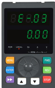
Fig. 4-5 Fault alarm display state
